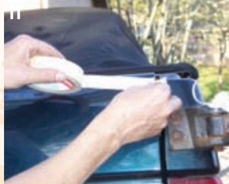
11 Then I placed a strip of masking tape along the tailgate centering it on the 6" line. Then drew a line across at the 6" mark.
