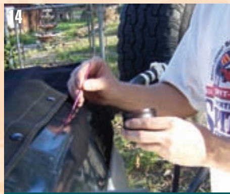
14 To stop rust in the future I dabbed a little Rust Bullet into the drilled holes. Any paint should do but I know Rust Bullet works!
