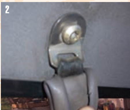
2 Then remove the seat belt anchor with the T-50...if your Bronco has shoulder belts.
