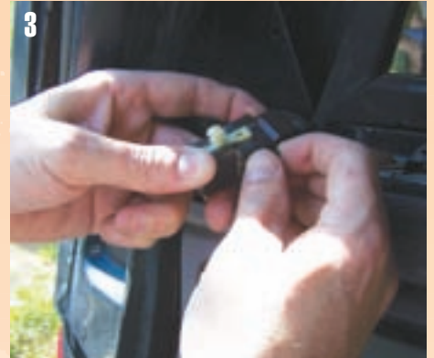
3 Unclip the third brake light connector (if applicable) located on the driver's side beside the tailgate.
