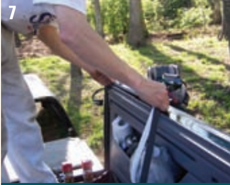
7 The first step is to put down the foam tape in the area where the brackets would rub the paint. Starting at the rear I worked my way around the perimeter of the truck.
