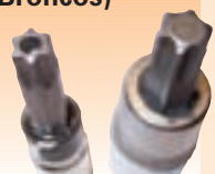
4 Now remove all the hard top bolts using the tamperproof T-40 bit or 8mm socket. The bolts are held to the body by "fender clips." Be sure not to let them fall into the body. Fishing them out is nearly impossible (don't ask how I know this).
