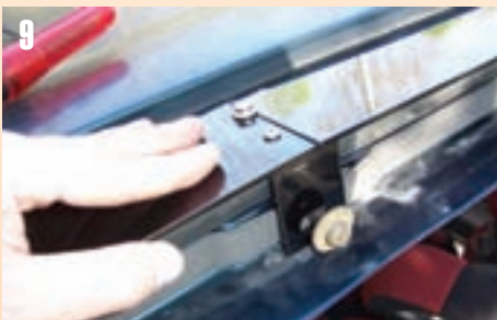
9 The two halves of the upper rail are connected together with two screws, one plain and one with a snap. Next, starting at the center, finger tighten the upper rail to the body with supplied bolts. The photo shows the factory bolt... I used supplied bolts AFTER the photo was taken. Now, attach the side rails to the body in the same manner... but use the factory bolts here.
