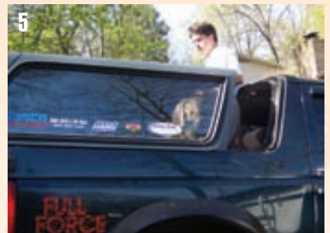
5 Now it is time to take off the top. This is at least a two man job, not too heavy but certainly is difficult to manoeuvre especially off a lifted truck. It helps to back up to a hill as I did so you won't have to bring it down so far.
