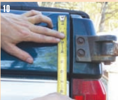
10 On to the tailgate. I measured up 6" from the body line and marked it. This is where the row of snaps will go.
