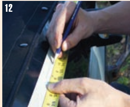
12 Next I measured to find the center of the tailgate and marked it. The remaining snap locations are 8 1/4" apart, four on each side starting in the center.
