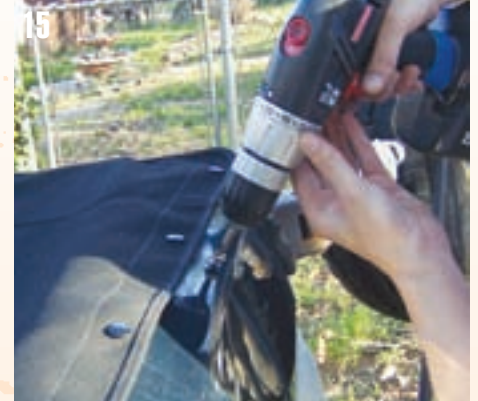
15 Next I screwed in the snaps to the tailgate. Done!
