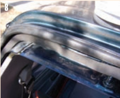
8 This is a closeup view of how the foam tape turns and covers the fender clips. I use a sharp tool to punch a hole in the tape (not shown) to allow the bolts through.
