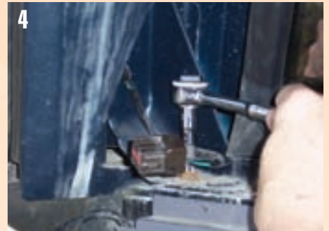
4 Now remove all the hard top bolts using the tamperproof T-40 bit or 8mm socket. The bolts are held to the body by "fender clips." Be sure not to let them fall into the body. Fishing them out is nearly impossible (don't ask how I know this).
