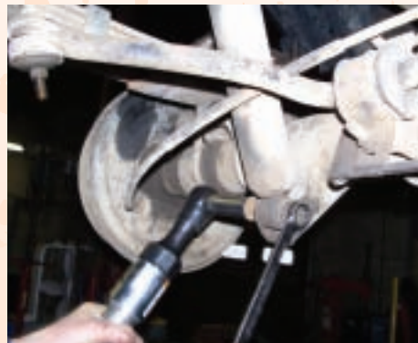
Moving to the rear suspension, the rear shock absorbers are removed.
