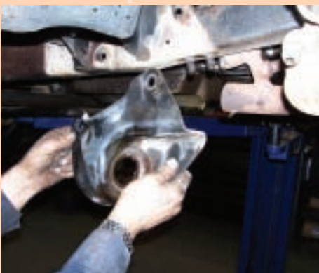
The stock radius arm brackets are removed.
