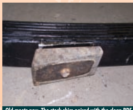
Old meets new. The stock shim paired with the clean BDS leaf spring pack. This stock shim positions the rear axle to maintain proper pinion angle.
