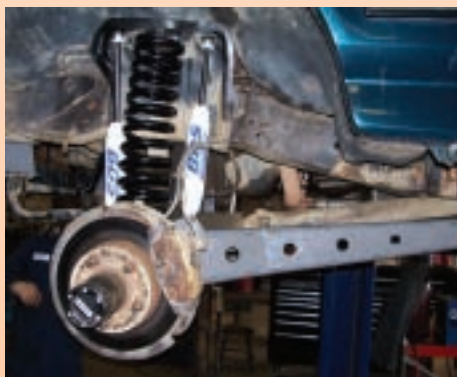
The BDS radius arms are a stout upgrade from the stock arms.
