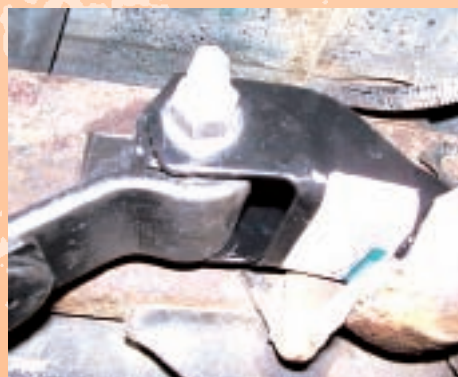
The new BDS leaf spring bracket is an improvement over the old, rusty components.
