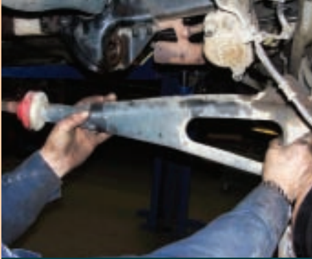
The radius arm is then disconnected from its rear bracket and removed.
