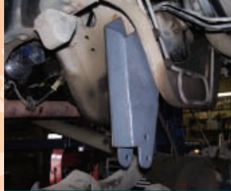
The BDS TTB drop bracket is installed on the passenger side.
