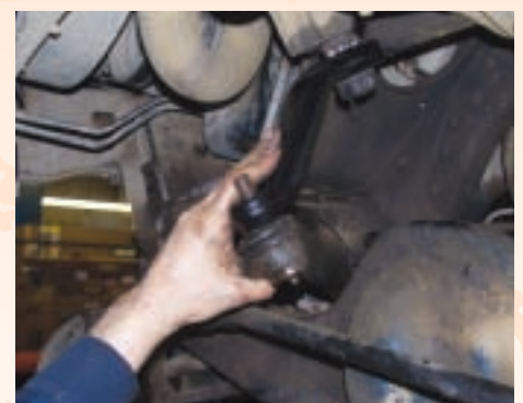
The dropped pitman arm is attached then the steering components.
