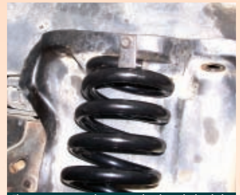
The new springs are then mounted and attached with the spring retainers.
