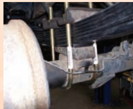
The rear BDS suspension now sits above the rear axle (looking forward on the driver side).
