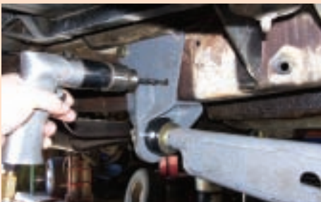
The new holes for the BDS radius arm brackets are drilled using the holes provided on the new bracket as a guide. It is important to take plenty of measurements before you begin in order to position the new brackets accurately and to maintain the front axle's original position after the new radius arms are installed.
